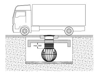
Cover heights for installation in groundwater - the hatched area shows the permissible submersion depth of the shaft, see also 6.2.2.
