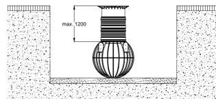
Cover heights with cast iron telescopic dome shaft (class B) in area driven over by vehicles up to 3.5 tonnes without groundwater or standing groundwater, see also 7.3.
